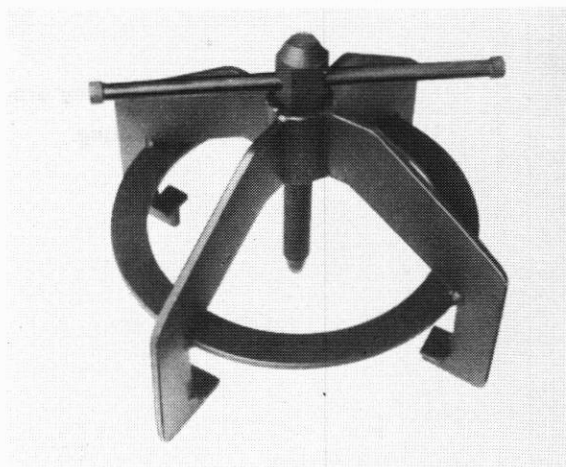
Extraction of front & rear brake drum.
